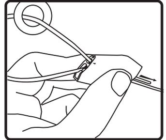
4. Thread cable end(s) through Gripple cable mechanisms as shown.
