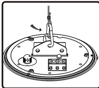
7. Attach snap hook by inserting one end through the hold on mounting bracket.
