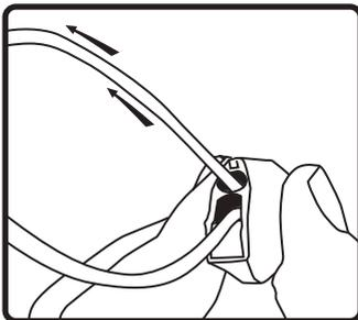
5. Adjust speaker hanging height with Gripple cable mechanism. Pull to tighten & press button on Gripple cable as shown to loosen or adjust.
