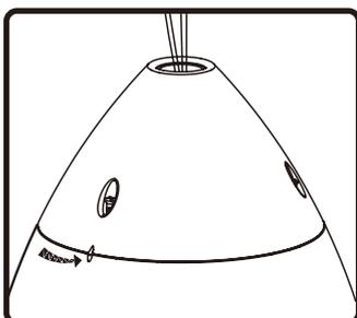
10. Place cover plate onto top of speaker and slightly rotate until alignment indicators meet.
